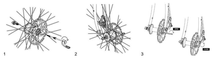
Step1: Install quick release to front hub.
