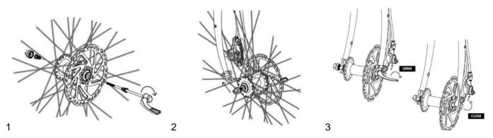
Step1: Install quick release to front hub.
