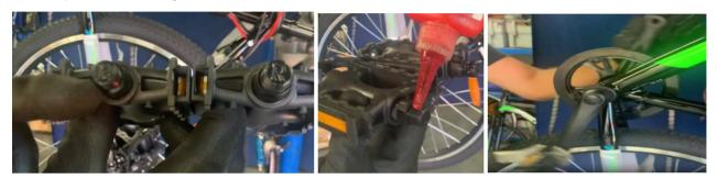
Note: Check if the pedals are loose before each ride. Applying LOCTITE is a good idea keep it secure.
