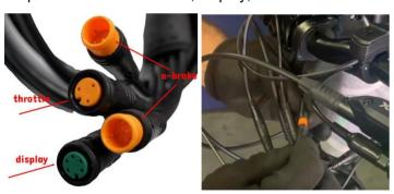
Note: DO NOT stretching the main cable (1 to 4) or have the cable caught by other bike parts. This may result internal electrical wire damage and have your warranty voided
