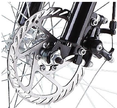
Typical Disc Brake
