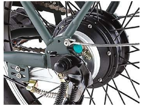
Typical Drum Brake
