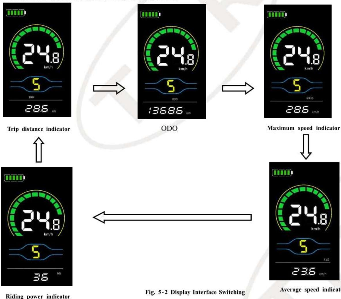
Fig. 5-2 Display Interface Switching
